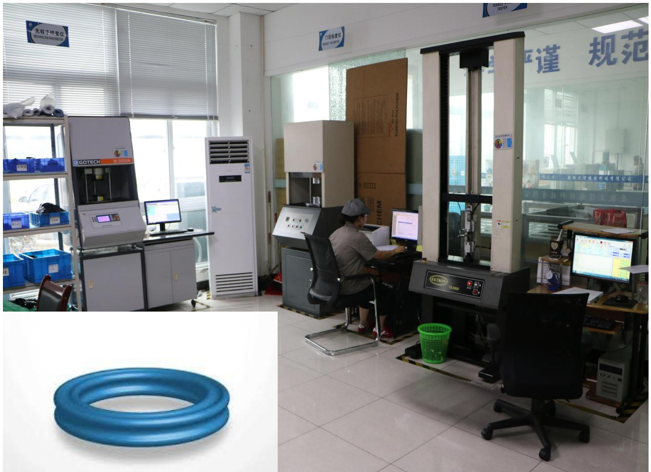
Another reason to choose an X ring for a dynamic application is that their structure prevents spiral twisting. The four ends of the X shape provide a stability that an O ring cannot offer. An O ring is perfectly adequate for some low-speed pivoting, rotating or spiralling movement, but an X ring can better accommodate faster motion. An O ring might do the job for a short period, but an X ring will be more durable in applications with rapidly moving parts.
